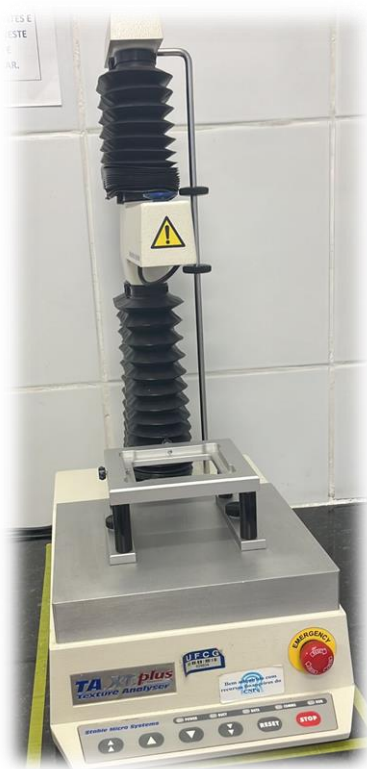
Figura 2 – TA.XT Plus Texture Analyser
