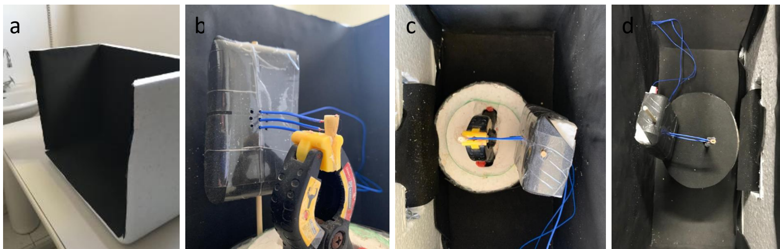
Figure 2. (a) Box of expanded polystyrene plates coated with aluminum foil covered by black Ethylene Vinyl Acetate (EVA). (b) Sample fixed with plastic pliers and thermocouple plugs - front view. (c) Sample fixed with plastic pliers and thermocouple plugs – upper view (d) Record of the temperature acquired by thermocouples by filming.
