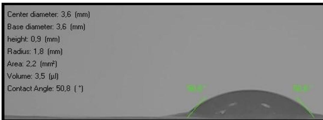
Membrana PA66/5% CaCO<sub>3</sub> para t=80s
